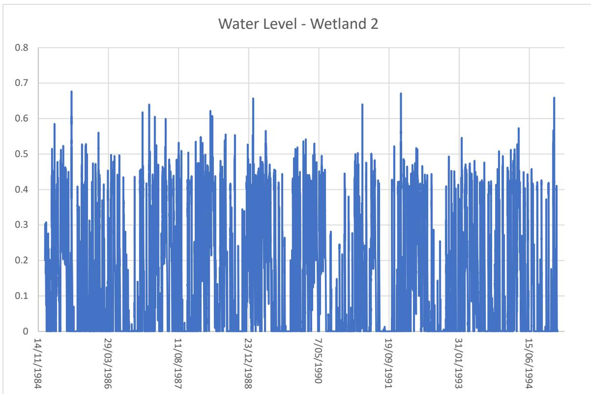
Figure 4 Modelled water level fluctuations in Wetland Cell 2 (1984-1994)
