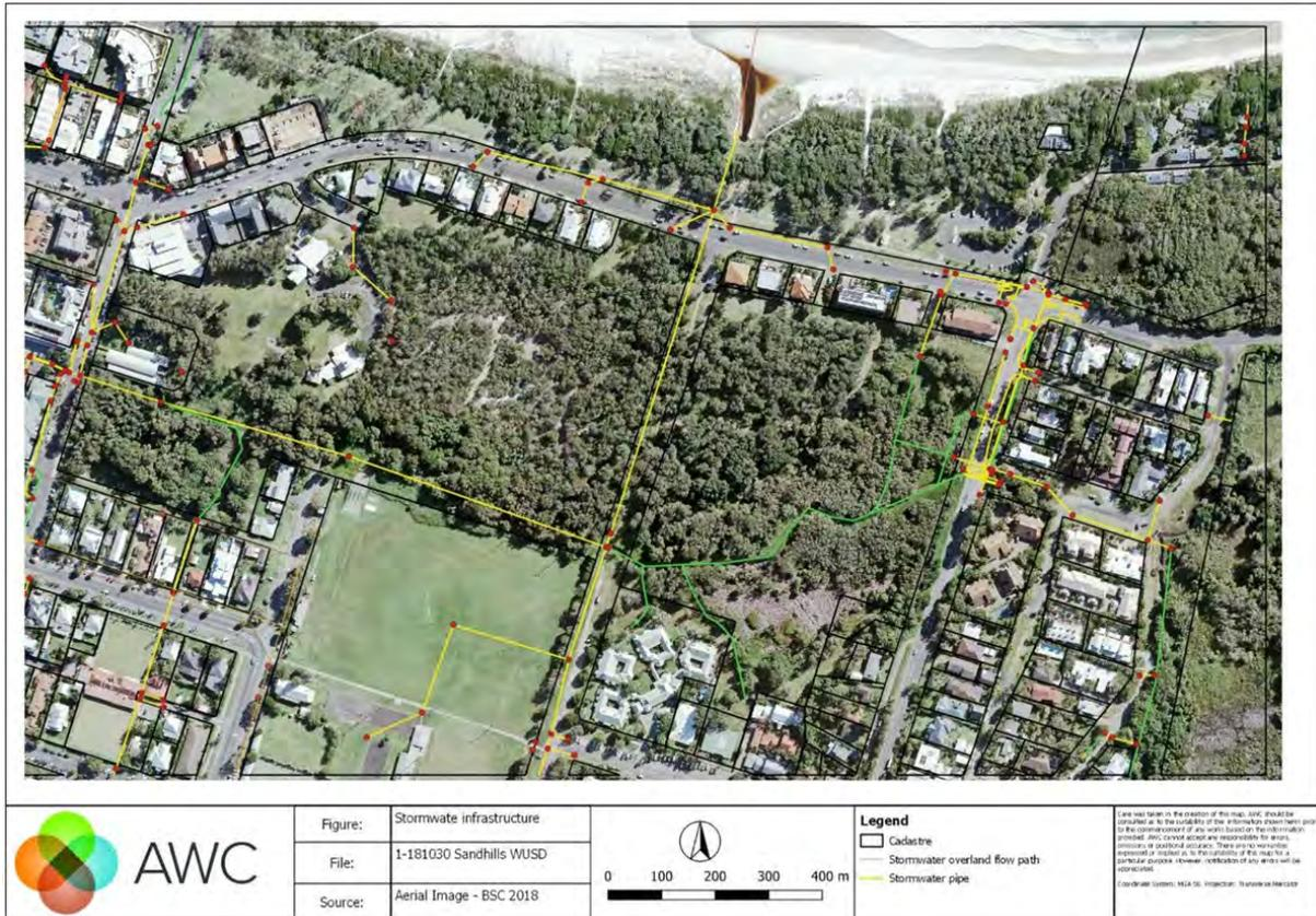
Figure 1 Stormwater infrastructure plan with piped network shown in yellow and surface system shown in green
