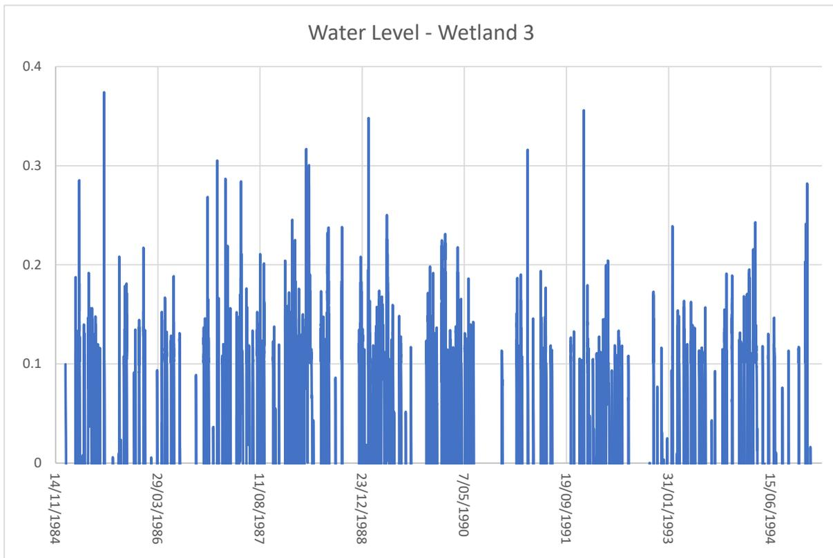
Figure 5 Modelled water level fluctuations in Wetland Cell 3 (1984-1994)
