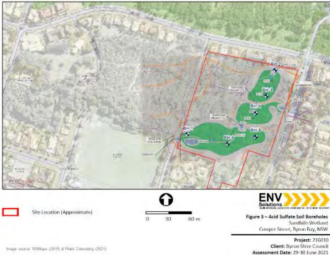
Figure 2 Acid Sulphate Soil Borehole locations overlain on the Sandhills Wetland Concept layout.
