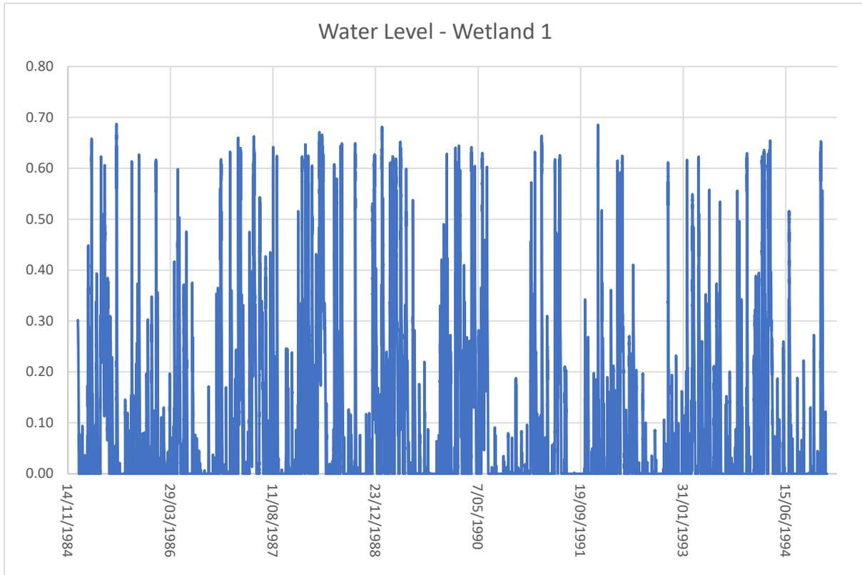
Figure 3 Modelled water level fluctuations in Wetland Cell 1 (1984-1994)
